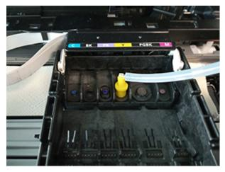
8. To fill the flushing hose, use a syringe with a needle and fill the hose halfway with nozzle cleaner. Then connect an empty refill syringe to the hose. Make sure the syringe plunger is pulled up slightly to allow air to enter the syringe body.
