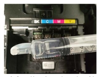
9. Start with gentle pumping motions of the syringe plunger to push the nozzle cleaner into the print head. The surfactants in the cleaner slowly dissolve clogs and dried out nozzles. Take your time and let the cleaner take effect.
