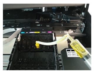
10. Be careful not to push too hard to prevent the plastic hose from pulling out of the ink inlet. Once the cleaner flows smoothly into the printhead, push one or two milliliters through the printhead. The escaping cleaner is trapped under the nozzle plate by the absorbent pad.
