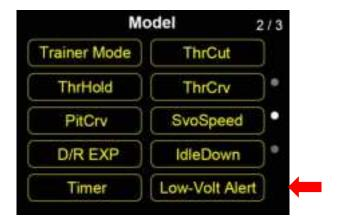
By using telemetry function, users can set a minimum voltage limit as safe level on FT24 transmitter, lower than which transmitter will send voice alert.
