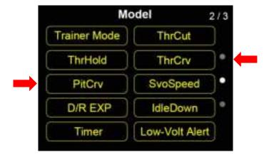
For smoother experience on operating throttle stick, FT24 supports up to 3 groups of curves, each group of which supports up to 6 points for adjusting.
