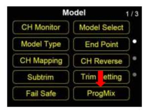
For some complex requirement of operating models, mostly helicopters and planes, FT24 transmitter supports up to 10 groups of programming and mixing. Linear control from 1 to 6, curve control from 7 to 10.
