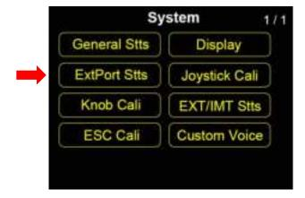
Expanding Ports function allows users to adjust FT24 transmitter outputting settings for supporting more external devices.
