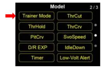
Trainer Mode (Master-Slave) helps experienced RC hobbyists train new talents. Under this mode, two FT24 transmitters can be linked through a trainer cable or be linked wirelessly. All channels are open for trainer mode, users decide which channel to use, and through a physical switch you can switch between master transmitter and slave transmitter.
