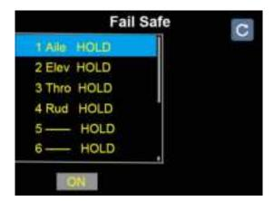
4. In Fail-Safe page, the function is default to be "OFF" and it displays "HOLD" in each channel. Under this configuration, if transmitter lost control to receiver, the
