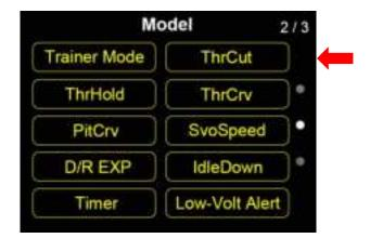
When Throttle Cut function is turned on, throttle channel outputs a fixed value. In this case, pushing on throttle stick does not output no value. Turn off the function to be back normal.
