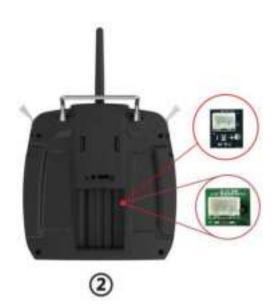
Mark: When you use a LiPo battery as power supply, please pay attention to the connector board and positive/negative definition. If the connector board is black, you can plug in 2S battery balancing connector directly for power supply. If the connector board is green, please follow the connector definition to make wiring.
