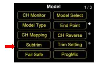
"Sub-Trim" page helps users set the middle position of channel output value and do trimming configuration to model/aircraft's flight attitude. Please make sure your target channel output is in middle position before doing "Sub-Trim".
