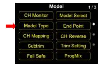
FT24 transmitter supports multiple model types. Planes, copters, gliders, multirotors (racing drones, agricultural drones, commercial drones), vehicles and boats, and robotics. Each model type has been configured in advance. Users can choose and make customized configuration.
