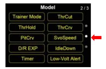
Servo speed function is designed to accomplish some special mission by adjust the changing ratio of an output channel. For example, it could be too fast to pack up or lay down landing gear in normal servo speed. So, we increase the channel's output ratio. Larger the value is, slower the channel outputs.
