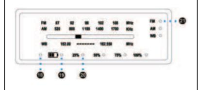
**®Working Indicator:** This indicator lights up when the device is working. Working status includes using: FM/AM/WB radio, flashlight, reading lamp, Bluetooth speaker.
