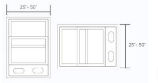
The window installation kit allows you to install the air conditioner in most vertical sliding windows 25" to 50" wide, or horizontal·s1iding windows from 18" to 50" high.
