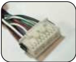
Interface Connector 2 (20-pin)
