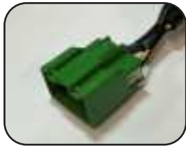
Vehicle Connector 1 (20-pin)
