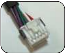
Interface Connector 3 (12-pin)
