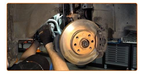
Screw the fasteners of the stabilizer bush brackets. Use a drive socket #E12. Use a torque wrench. Tighten it to 35 nm torque.
