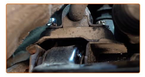
Unscrew the fasteners of the stabilizer bush brackets. Use a combination spanner #13.
