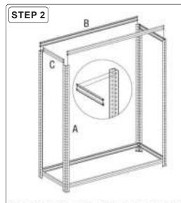
Fasten Short Beams (Part C) to the top of the Angle Posts (Part A) as shown, followed by Long Beams (Part B) to opposing kayholes to form the frame. NOTE: Flat edges face outwards. Lock rivets to the bottom of the kayhole by tapping the Beams with a Rubber Mallet.
