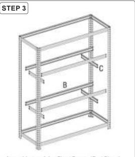
Assemble remaining Short Beams (Part C) and Long Beams (Part B) to your desired shelf height. As before, lock rivets to the bottom of the keyhole by tapping the Beams with a rubber mailet.
