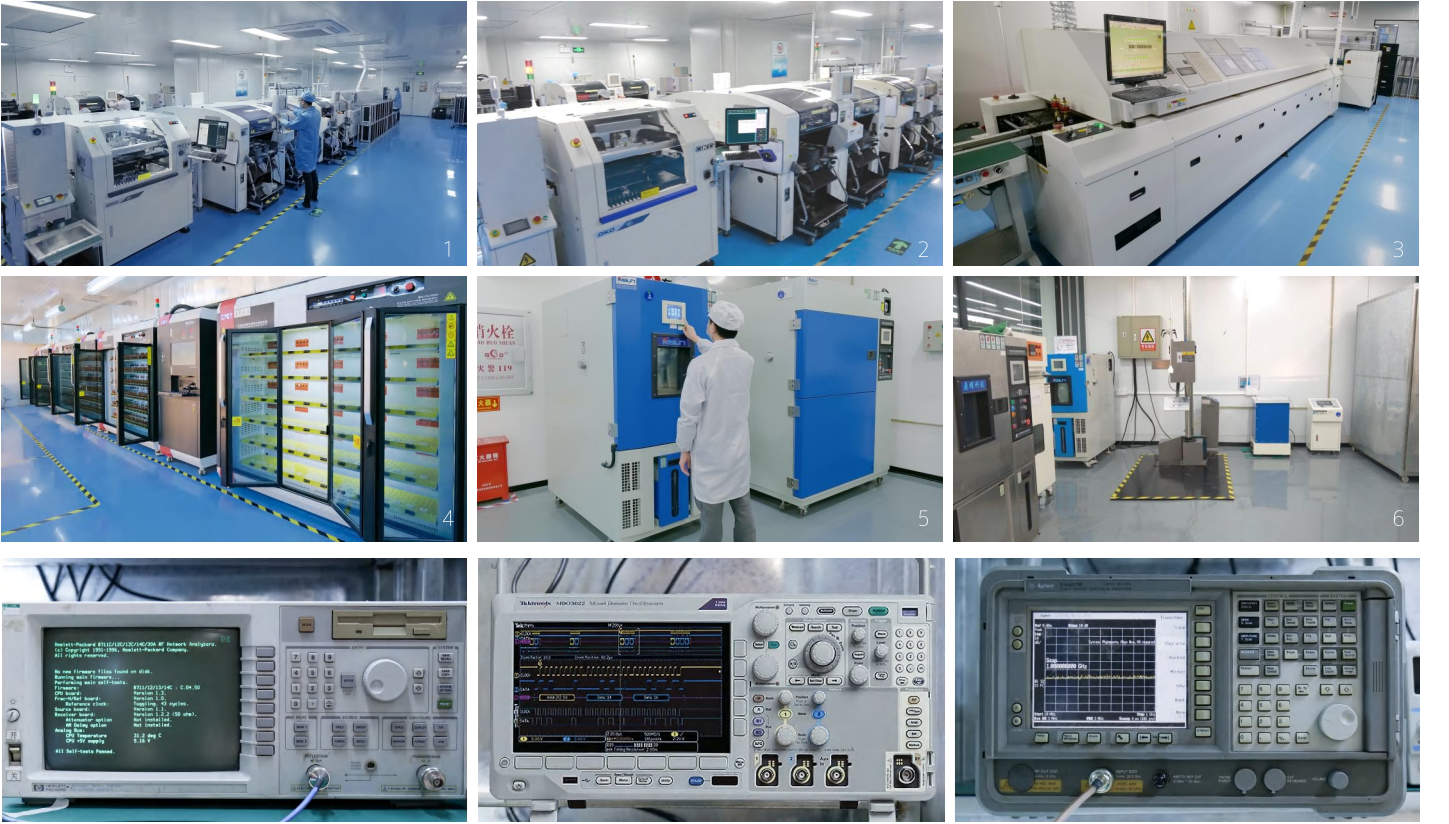
1. SMT Workshop 2. SMT equipment 3. Reflow soldering 4. Aging equipment 5. Temperature test 6. Drop Test 7. Network analyzer 8. Oscilloscope 9. Spectrometer
