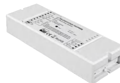
Model Input Voltage Input Current Output SR-ZV9101FA(0-10V/PWM) 100-240Vac 60mA 2x(0-5V), 2x(0-10V), 2x(0-15V)
