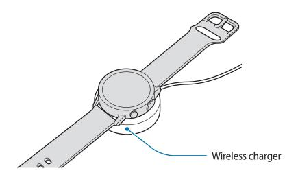
3 After fully charging, disconnect the Galaxy Watch Active2 from the wireless charger. First, disconnect the wireless charger from the charger and then unplug the charger from the electric socket.
