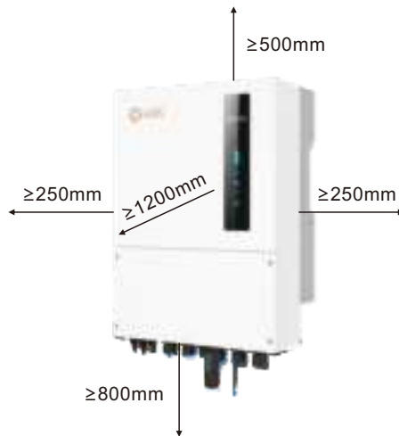
Figure 3.5 Inverter Mounting Clearances
