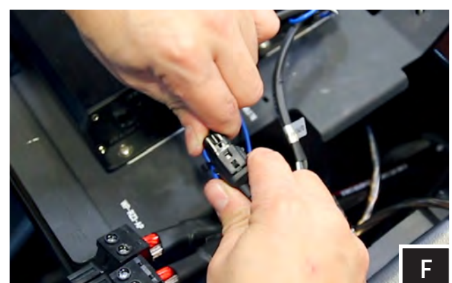
F. Connect the B-H1149 speaker harness to the amplifier front output (white/grey).
