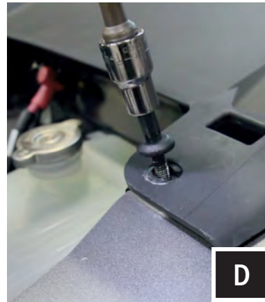
D. Remove center dash by unscrewing the 2 T-30 Torx screws and push center dash forward to unclip.
