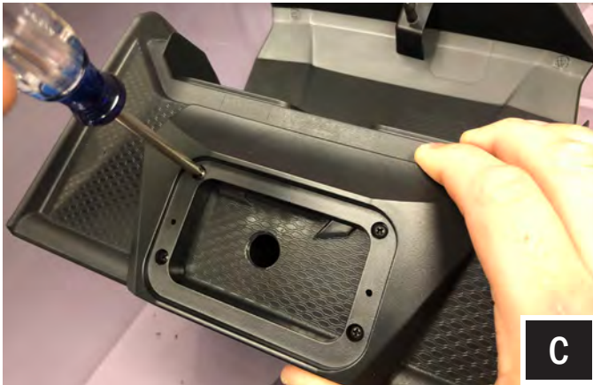
C. Align DM3 over drilled holes on the compartment. Secure the DM3 to the compartment with (4) of the provided MRB3 dash screws. **Do not over torque**
