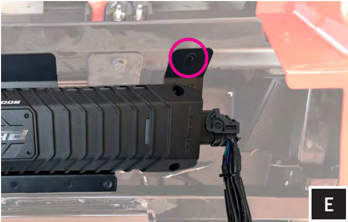
E. With the accurate location marked, uninstall the amp tray and use a 13/64" drill bit to drill your pilot hole. With your pilot hole drilled, reinstall the amp tray. Use the self-tapping screw in the drilled hole location.
