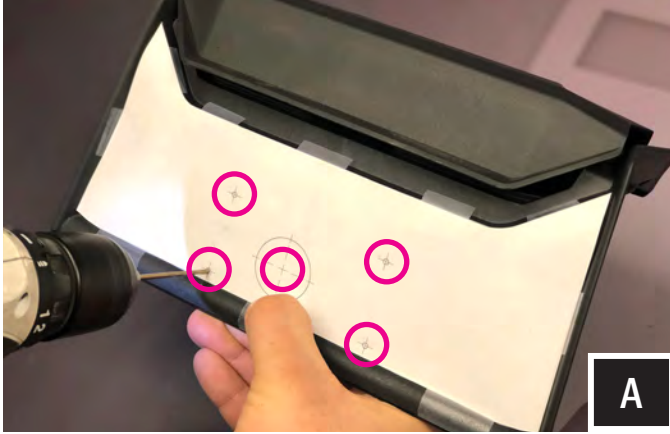
A. Using a 3/32" drill bit, drill out each template guide point and a pilot hole into the center guide point.
