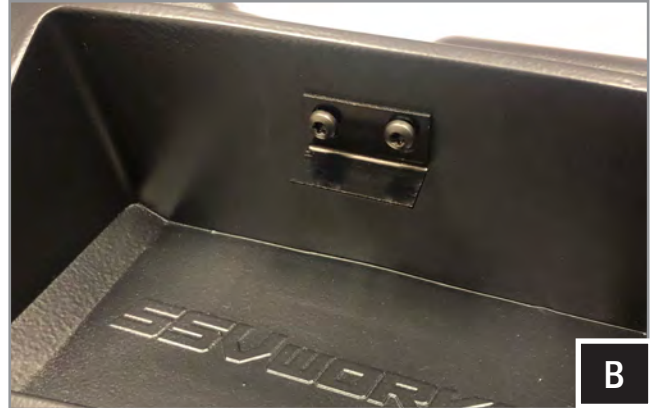
B. Install door latch onto enclosure with the provided (2) T30 M6x8mm screws.
