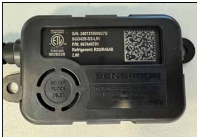
FIGURE 14. Example of Clear, Unobstructed Sensor Inlet
