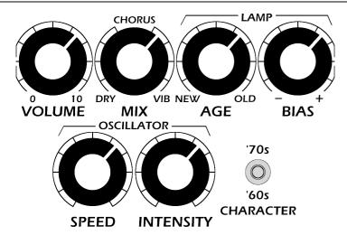
**VOLUME:** Increases the output volume level as the knob is turned clockwise.
