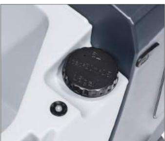
2. Fill the solution tank with clean water. The clean water temperature must not exceed 40 °C.
