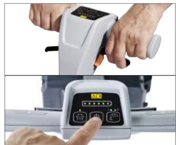
4. Adjust the handle to the desired height. Turn on the machine with the main button.
