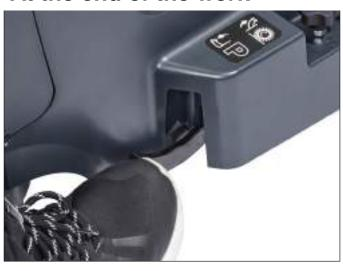
11. For the transportation and the parking of the machine, push down the pedal (slightly lift the front of the machine by tilting the handlebar).
