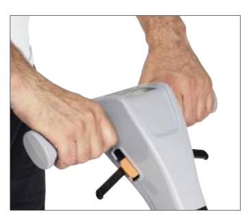
6. Grab the handles to activate the brush and solution flow, then start cleaning the floor.
