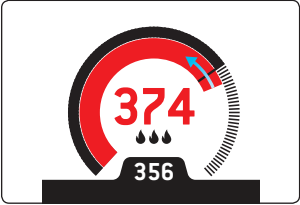
Cooling to set temperature.
