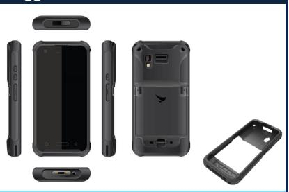
CF550 Rugged boot protects the mobile computer from wear and tear, providing more ruggedness at the same time.
