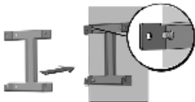
Figure 12: Placing bracket onto wall anchors
