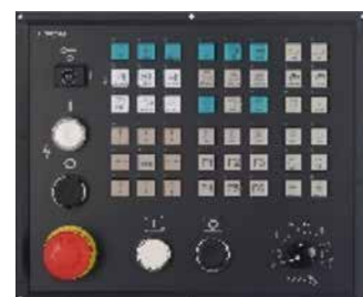
Control Panel for Mill
