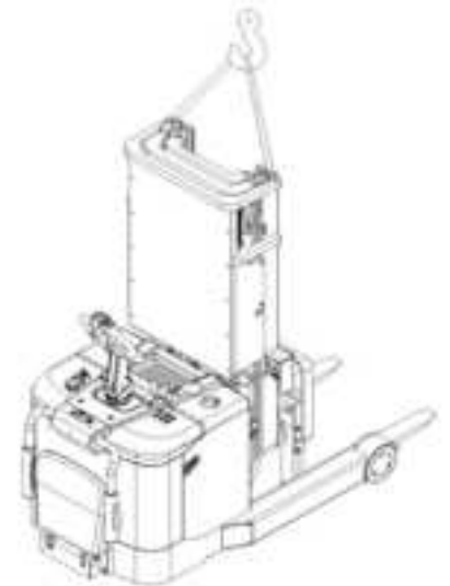
Fig.5: Lifting with a crane
