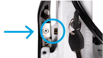
Locking Pin protruding through frame
