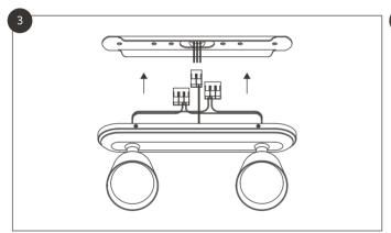
Using the terminal box provided, connect the live (brown) and neutral (blue) wires. Tuck the wires and the terminal box into the void. Push the brass cover over the mounting plate.
