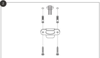
Use the screws and anchors provided to attach the mounting plate to the ceiling or wall.
