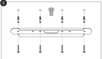
Use the four screws and anchors provided to attach the mounting plate to the ceiling or wall.
