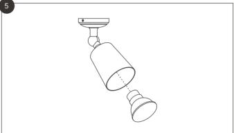
(Court) into the shade and test the light to make sure the wiring is correct.
