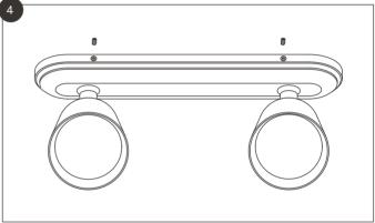
When the cover is flush with the ceiling or wall, tighten the four grub screws to secure the spotlight.
