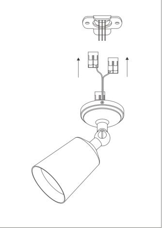
Using the terminal box provided, connect the live (brown) and neutral (blue) wires. Tuck the wires and the terminal box into the void and push the brass cover over the mounting plate.
