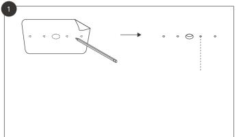
Drill the 20mm hole for the wires and the four 6mm holes for the plastic anchors. See template on **page 6.**
