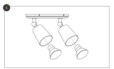
Insert 50mm GU10 bulbs (Arthur or Chester) or 35mm bulbs (Court) into the shades and test the light to make sure the wiring is correct.
