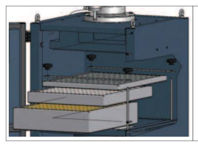
In the case of panel filters, loosen the 4 knobs so that the 2 filter fixing crossbars can be raised.
