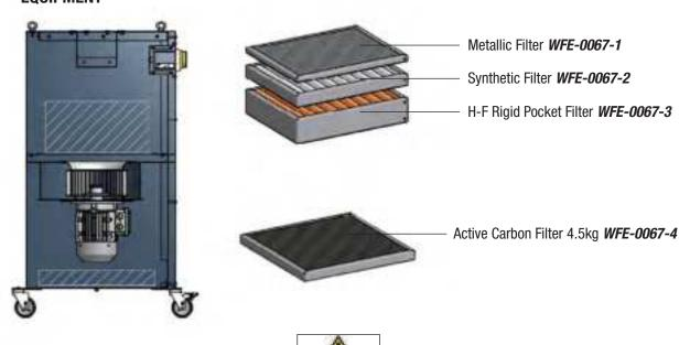
**Important:** when servicing machines equipped with panel filters, strictly follow the sequence of filters shown in the diagram.
