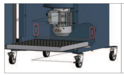
In the case of activated carbon filters, located in the lower compartment of the machine, loosen the 2 fixing screws shown in the figure so that the filter holding crossbar can be raised. Now lift the filter and remove it from its compartment.
