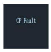
4.3 CP Fault: The device detects that the CP voltage exceeds  $6V \pm 0.8$  or  $9V \pm 0.8$ , reports a CP fault, recovers the voltage to within range, and recovers the fault.
