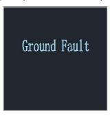
4.2 Ground Fault: The ground wire is not connected or the ground wire is poor.
