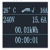
2.3 After inserting the charging gun head into the vehicle charging port, the charging interface is shown below:
