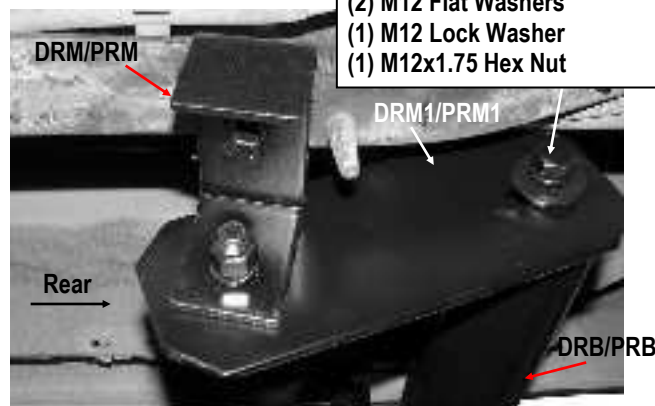
(Fig 7) Passenger Rear Bar Bracket Installed
