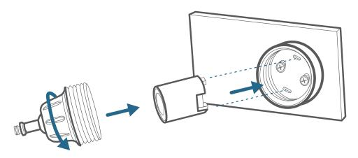
4. Screw the camera onto the mounting bracket. Position the camera to achieve the desired view, checking it using the live stream in the eufy Security app.
