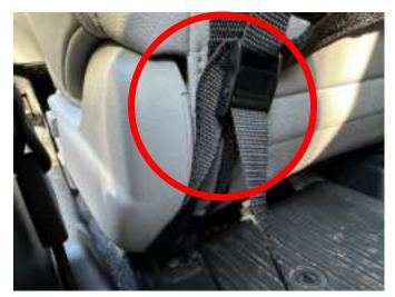
Tighten the top straps as desired while maintaining desired range of motion for the front seats. Finally draw the bottom straps tight just enough to not pull down the net past desired height position. Cover up the buckles and wrap up excess adjusting strap:
