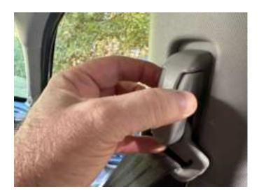
Press the lower panel into place ensuring that all tabs line up correctly.
