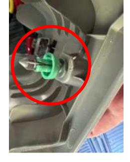
Slide the whole clip assembly down and out of the upper panel cover.
