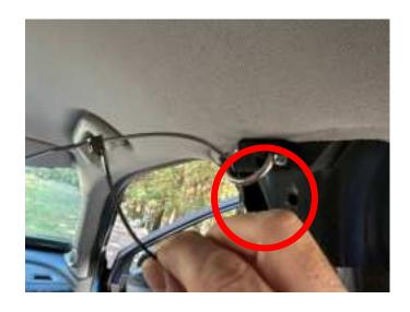
Remove the clip from the previous step by sliding down and off of the trim cover. You can then lift the side tabs of the green piece from the metal insert and reinstall the green receptor back into the B pillar opening hole:
