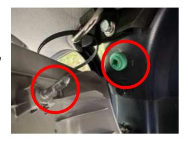
Keep the D ring up and clear of the trim cover and press into position
