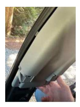
The service manual says that this clip should be considered a "one use" clip and to use a rubber mallet and a towel to tap it in, breaking off the profusion tabs.
