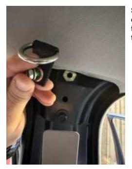
Slide the C100G hardware piece supplied with your net onto this bolt. Reinstall and finger tighten to start the threads and then twist the tether and D ring oriented to the top:
