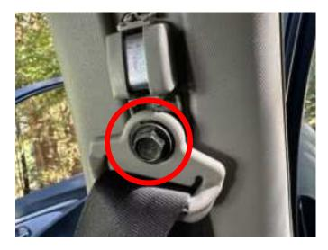
Ensure that there is no restriction with the seat belt webbing and reinstall the adjuster cover:
