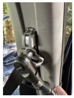
Remove the exposed 14mm bolt securing the upper seat belt adjuster:
