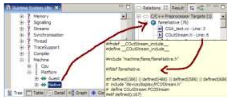
Figure 7. Representation of a C/C++ Preprocessor Constant in the Relations View
