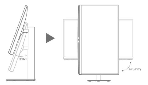
Erect the monitor, adjust the height and tilt angle of the screen to the maximum, face the screen, and rotate the screen 90 degrees clockwise until the screen is in portrait mode.
