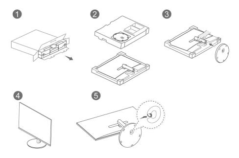
1 Place the carton horizontally with the foam arrow facing upwards, open the carton, and take out the device and foam.
