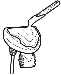
Applying Epoxy to the 200/83 kHz Transducer
