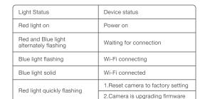
NOTE: The device is hibernating, and the indicator light turns off. To check if the device is powered on, click the reset button to see if the indicator light is on.
