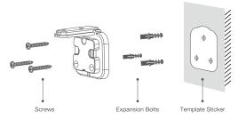
1. Take out the bracket and accessories, Choose a proper installation location, and make holes according to the positioning sticker. Install the rubber plug and tighten the screws to firm the bracket .
