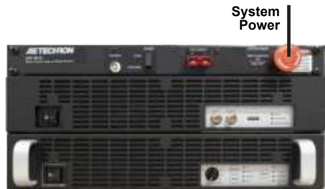
Figure 2.6 – System Power Switch Location
