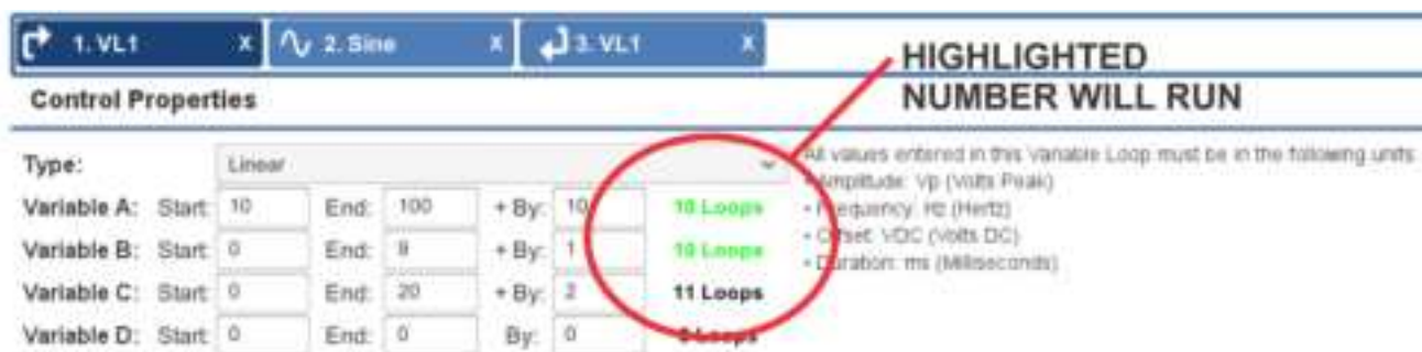
Figure 6.11 – Adding Additional Variables to a Linear Variable Loop
