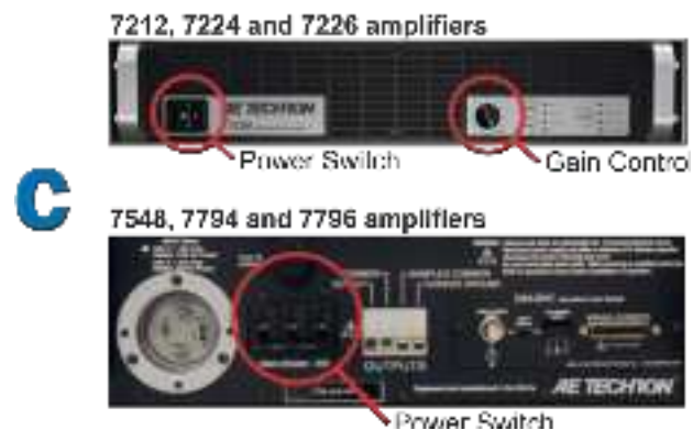
Figure 2.5 – Amplifier gain control and power switch.
