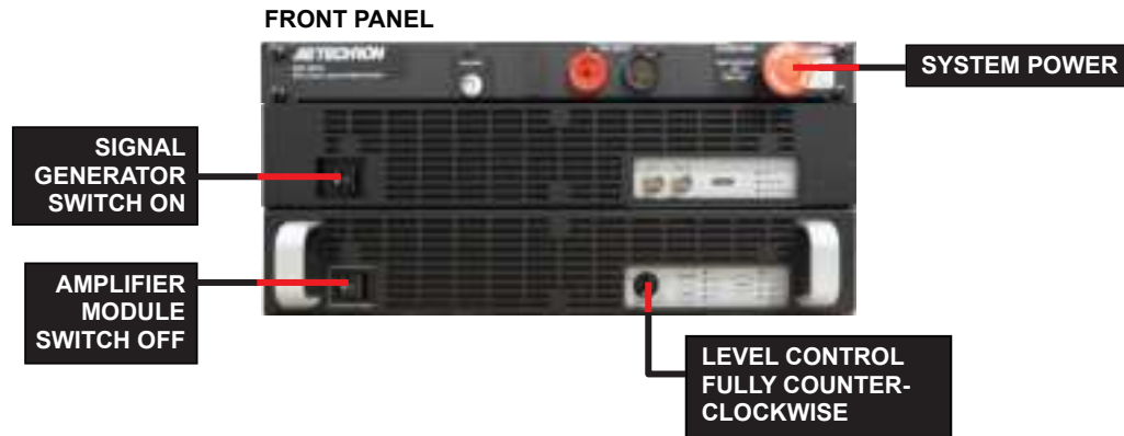
Figure 4.7 – Locations of Controls for Operation with an External Amplifier
