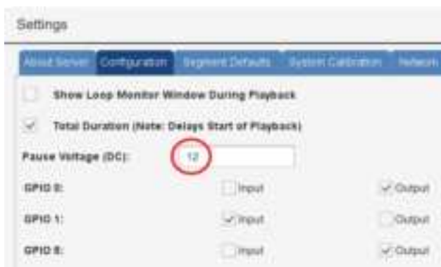
Figure 5.15 – Setting the Pause Voltage (DC)
