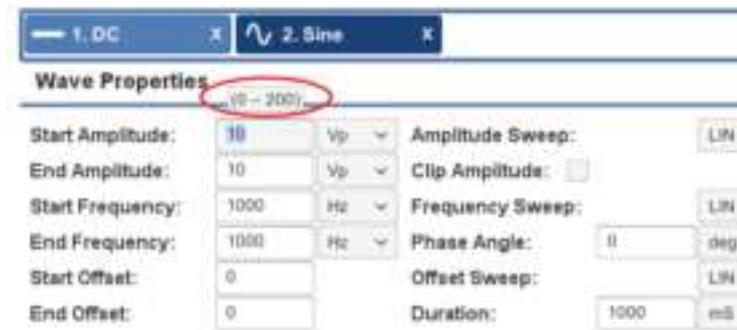
Figure 5.10 – Viewing the allowable range for a waveform property.
