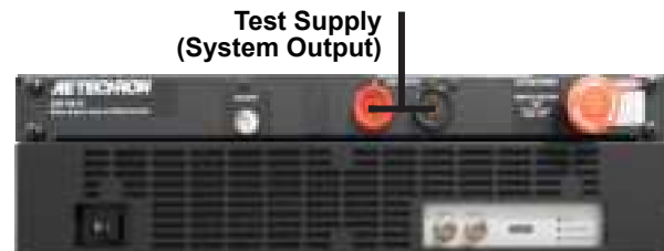
Figure 2.2 – Test Supply Connectors
