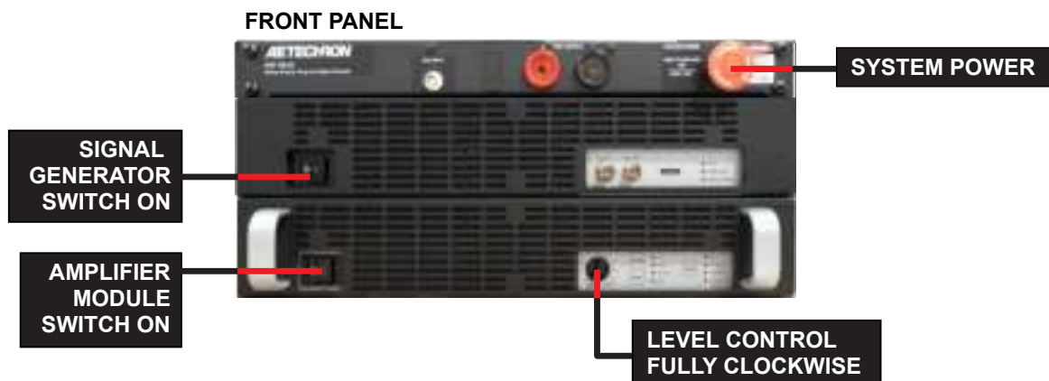
Figure 4.3 – Locations of Controls for Low-Voltage Testing
