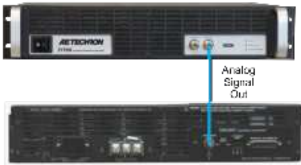
Figure 2.2 – Connecting an amplifier to the 3110A
