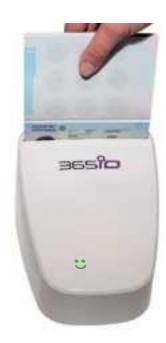
If you remove the passport too early or touch it during the scanning process, the result may be incorrect (yellow or red indication). If so, remove the passport and start over.
