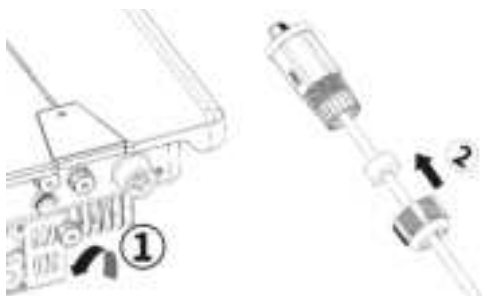
Fig. 31 Configure Network cable
