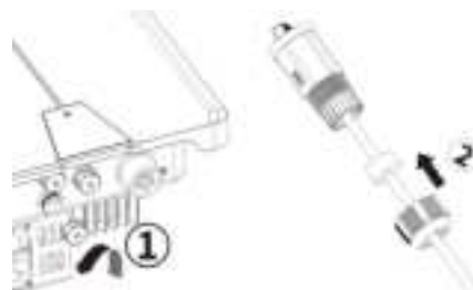
Fig. 28: insert the network cab
