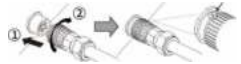
Fig. 18: Engage the AC connector with the device connector
