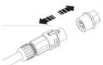
Fig. 39: Detach the AC connection plug Fig. 40: Disconnect AC connection plug Fig. 41: Release the cable
