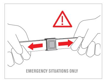
In the event of an emergency where removal of the BMT is required, pulling the neck strap apart in opposite directions will quickly disengage the clasp.
