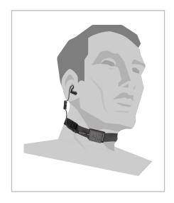
II. Place the throat mic around your neck and reapply the clasp so that it makes contact. The optimal position for a throat mic is about 1-1.5" to the side of the voice box where the BMT is positioned.
