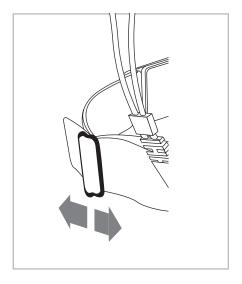
III. Adjust the neck strap for tightness by using the adjusters (A2). The throat mic needs to be just snug but not tight around your neck.
