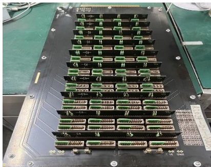
5.6: Small PCB on HTRB Board
