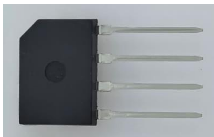
5.24: Through-hole sample before solder dip
