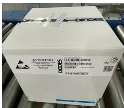
4.3: Inner box with MSL1 packing
