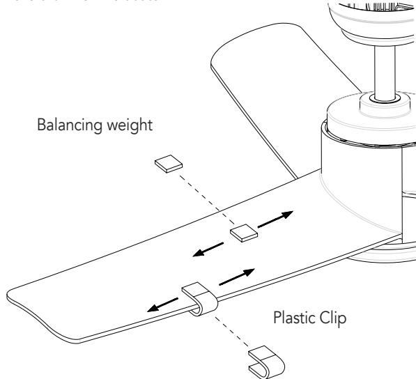
Turn on the fan and set the speed (usually high speed) that causes the worst oscillation.
