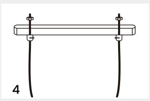
Thread the wires through the accessories that fix the wires and exit from above the ceiling panel. Secure the top with a nut and tighten the transparent screw that fixes the wires below.
