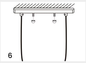
Screw through the ceiling plate and tighten with a nut
