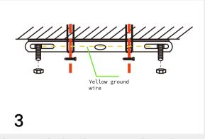
The ground wire is connected to the screw and connected to the household ground wire.
