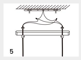
Tie the wires of the same color tightly with insulating tape
