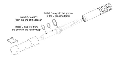
3. Install two O-rings onto the MX801 logger (see above). The O-rings serve to stabilize and center each part of the assembly.
