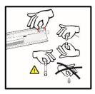
When handling the UV lamp, avoid touching the glass element with exposed fingers.
