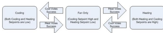
Figure 28: Changeover Voting State Diagram
