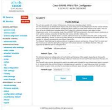
The following image shows, both radios must be configured as Fluidity for role Vehicle. if one wireless interface is configured in fixed mode and the other one is configured in Fluidity mode then unit role Vehicle cannot be selected.
