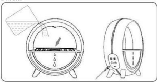
Power Button: Press and hold for 3 seconds to tum on or off the humidiier and the ambient light, and the humidifier starts to pump water and spray.
