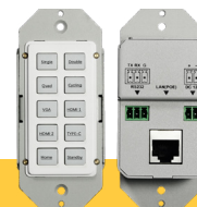
10-key Configurable control keypad Model: iCon-10-US, iCon-10-UK
