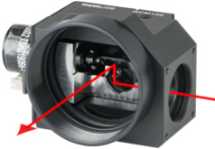
Beam Path Shown Through the Input Port, Reflecting off Both Galvo Mirrors, and then Exiting Through the SM2-Threaded Output Port
