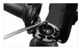
Use the included 5# hexagonal wrench to tighten the aluminum cover screws, and use the included hexagonal wrench to fix the screws on both sides of the riser.
