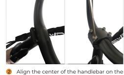
Align the center of the handlebar on the riser, make sure the left and right sides are symmetrical, fix the top cover with the screws, and tighten the four screws evenly.
