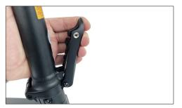
Press down the riser lock handle to lock the folding device.
