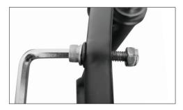
1 Use the Allen wrench and a wrench from the accessories kit, remove the screws and anti-skid nuts on the front fork hanger.
