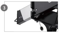
Withdraw the key and carefully pull the battery out from the frame.
