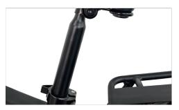
Insert the seat tube into the hole in the frame's center tube. Adjust the saddle so that the seat tube's head tube is parallel to the frame's top tube.
