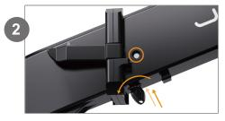
On the right side of the e-bike, press the key inward and simultaneously rotate it to the left until the button recesses.
