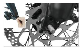
Remove the rubber plug on the disc brake and place the front wheel on the front fork (note that the disc is on the left side of the front fork)
