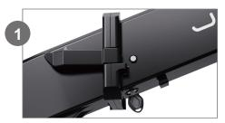
Open the frame quick-release lever and fold the bicycle.
