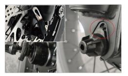
Then put the removed nut, safety hook gasket and spring together in turn, align the safety hook gaskets on the left and right sides with the round holes, and close the quick release handle with your palm or fingers. The locking force of the handle is 15-20kgf.cm to prevent the quick release from loosening during riding.
