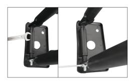
1 Fix the vehicle body and remove the front fork protection rod using the wrench in the accessory tool.
