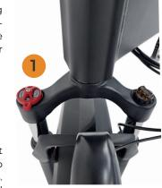
The lockout lever (1) ,located on top of the right side of the suspension fork, can be turned counterclockwise until it stops to completely lock out the suspension fork's travel. To unlock the lockout lever, turn the knob clockwise until it stops. When the lockout lever is unlocked, resistance can be adjusted by turning.
