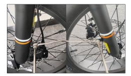
4 Fix the mud plate left side support to the left side of the front fork with the screw, then tighten.
