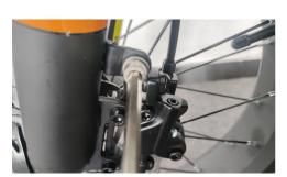
3 Use the included Allen wrench to remove the screws on both sides of the front fork.
