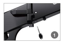
On the right side of the e-bike, insert the kev into the lock hole. now the e-bike is
