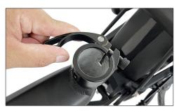
Hold the quick release handle with your hand and pull it outward to fully open it.
