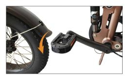
3 Gently screw the left pedal onto the left crank by hand, turn it counterclockwise, and then tighten the pedal with an open-end wrench.
