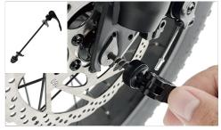
3 Remove the nut, safety hook gasket and spring of the front wheel quick release in sequence. Pass the front wheel quick release rod through the front hub axle core hole from the disc brake disc side. Be careful not to move the safety hook gasket and spring in sequence.
