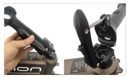
Put the seat tube onto the front fork vertical tube, unfold the folded seat tube, first use your thumb to lift the lock buckle upward without loosening it, then use your index finger to pull the seat tube outward to unfold it.
